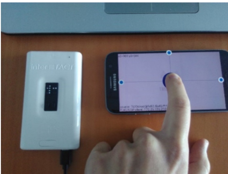
Figure 2 : A pin's configuration on the MIT5 according to the finger's position on
